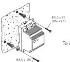
The power supply must be installed in a dry and protected place. It's recommended to protect the power supply by using a thermo-magnetic circuit breaker.
