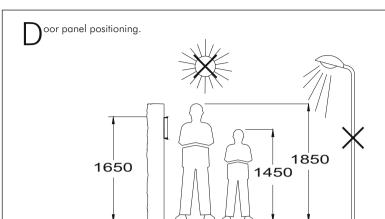
The upper part of the door panel should be placed at 1,65m.
