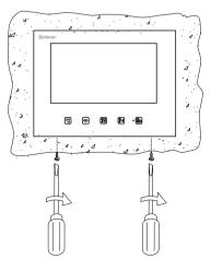
With help of an screwdriver, fix the monitor with especified screws, as shown on the picture.
