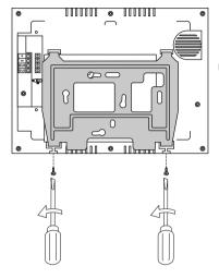
Unscrew the monitor bottom screws.
